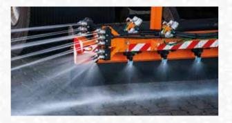
applied. Working widths of up to 15 metres can be achieved with fan nozzles and point steel nozzles, which can also be switched asymmetrically. This makes it possible to completely treat inlets, turning lanes, bus stops and intersections in just one pass.
