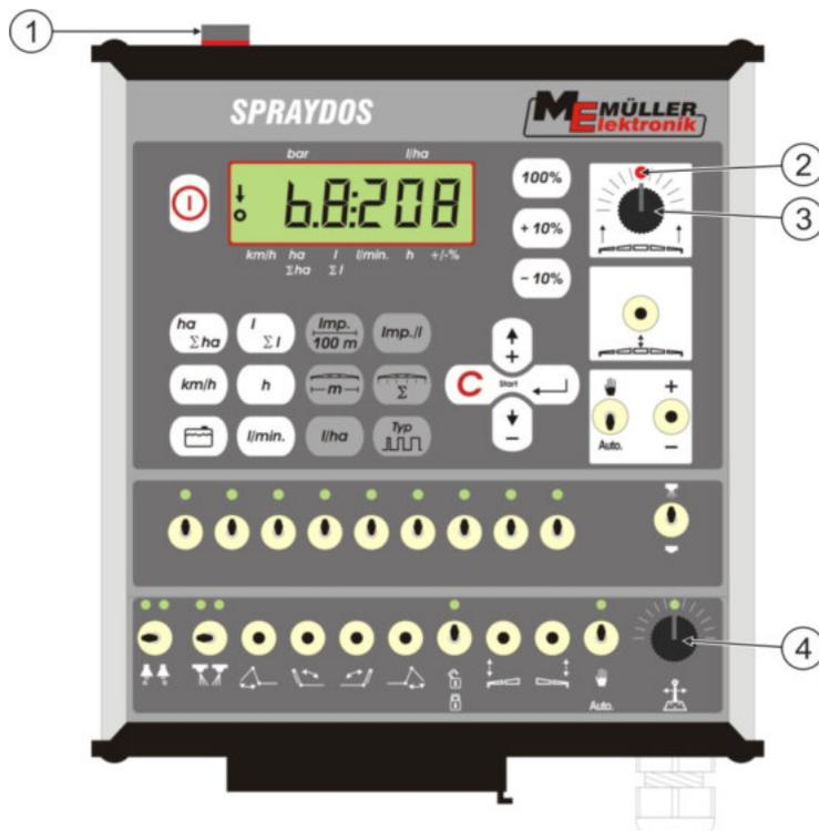
**Diagram 6-3 Operating elements that are required for calibration**
