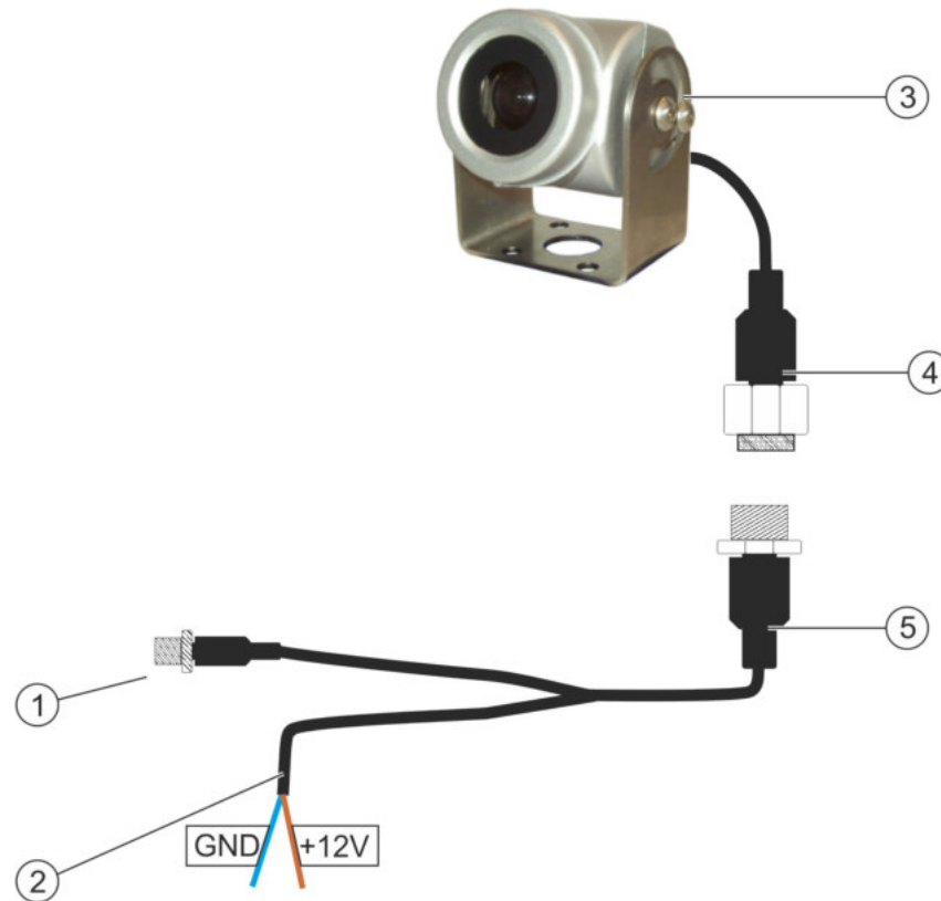
Camera with cable harness
