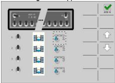
⇒ You can see which switch of the S-Box has been assigned to an ISOBUS job computer function. With the keys, you can view the assignment of the other switches.
