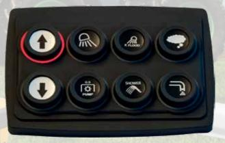
The new keypads make it easier to operate the built-up crop protection sprayer. The keypads are positioned in the immediate vicinity of the dispensing center so that the operator has the switching functions available outside the cabin. This additional user-friendliness of the crop protection syringe is available in two versions: the 4-key ESZ keypad and the 8-key sprayer keypad.
