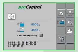
Canister flushing ☑ = Washing programmes can be interrupted
