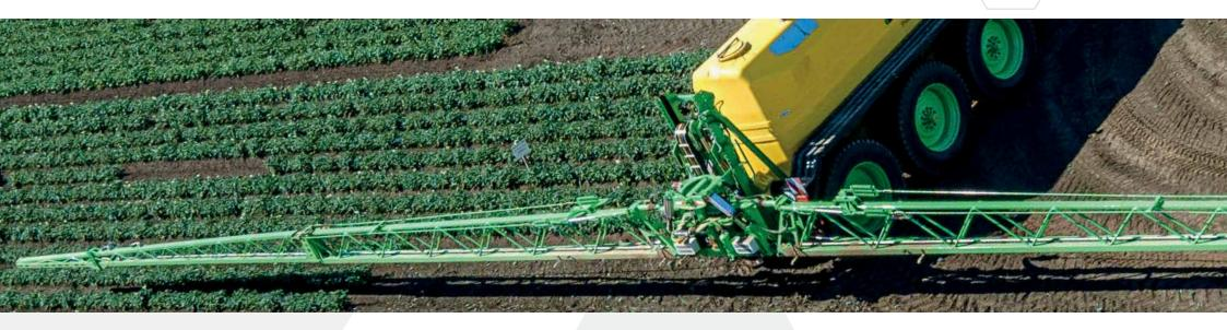
At the heart of the Profi-Class Tridem lies a three-axle, air-suspended chassis featuring mechanical-hydraulic forced steering for the first and third axles. This design offers excellent road holding and comfortable handling, particularly when the 20,000-litre tank is full. The K80 ball head coupling ensures reliable power transmission and maximum driving safety, even when travelling over uneven ground or performing fast manoeuvres.
