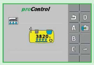
A/B/C/D button – freely configurable additional functions
