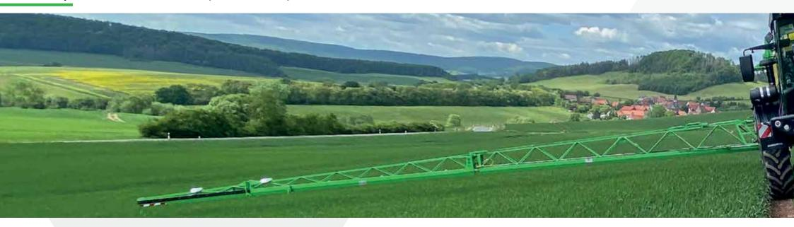
The **DAMMANN AgriBalance** is an innovative automatic system that actively guides our field sprayers. It ensures the boom is always at the optimal height and angle above the crop, even on uneven terrain or when the carrier vehicle is in motion.
