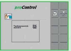
For example, it is possible to start the cleaning programme manually despite a defective tank sensor.
